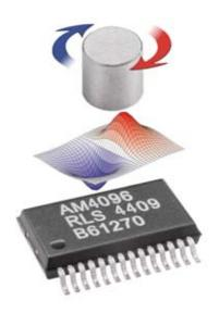
All of the sensor and processing electronics have been placed within the compact silicon design. The rotation of a simple north / south magnet is picked up by the AM4096's sensor and provides absolute positional information output.
